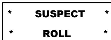
To view the amount estimated to be in a suspect roll, you can press coin **<↑>** or **<↓>** until the relevant denomination is reached. It may be, however, that the problem is not a missing or extra coin but one of the wrong denomination so it is advisable to split the roll, place the coins in a cup and count in loose coin mode.
