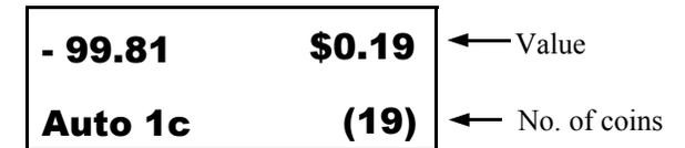
If **Auto Add is off**, leave cup on the tray and press <+> to add to the total,; remove the cup from the tray then press coin <↑> to move to the next denomination.
