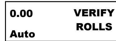
Simply apply one roll at a time, and wait for the Omega “C” to verify the roll before applying the next. You do not have to remove the previous roll before adding the next one.
