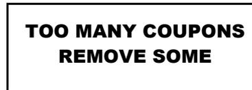
Although it should be possible to apply up to 35 at a time, the “**TOO MANY BILLS/COUPONS - REMOVE SOME**” message will be displayed more frequently if bills/coupons are in poor condition to those counted previously e.g. if counting brand new bills after very old ones. Simply remove a few bills/coupons from the cash tray until the error message disappears, then continue counting.
